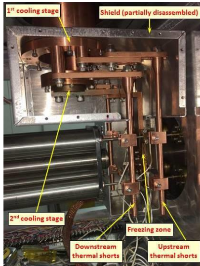
Fig. 3. The new cryostat configuration with added upstream and downstream thermal links to the first cooling stage
