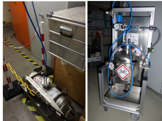
Fig. 6: Storage vessel and handling tool for mercury transfer.
