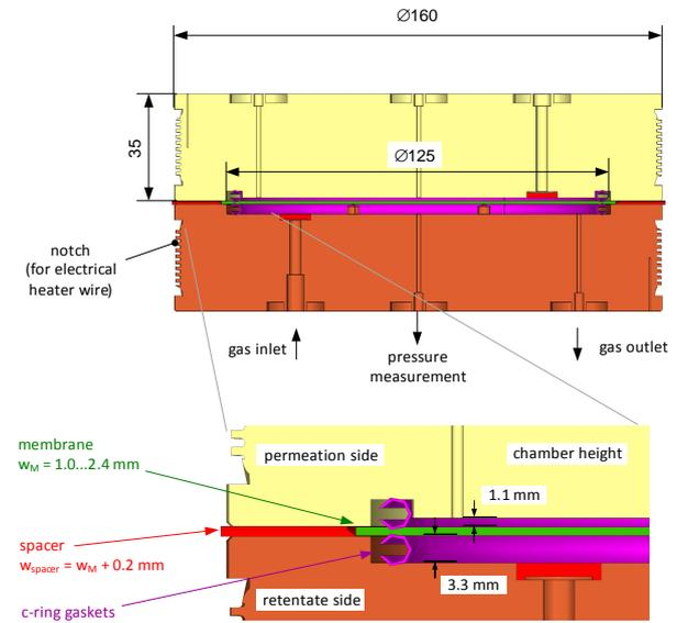
Fig. 2. Permeator composed of retentate side chamber and permeate side chamber separated by the permeation membrane. Top: overall view. Bottom: detail view with gaskets
