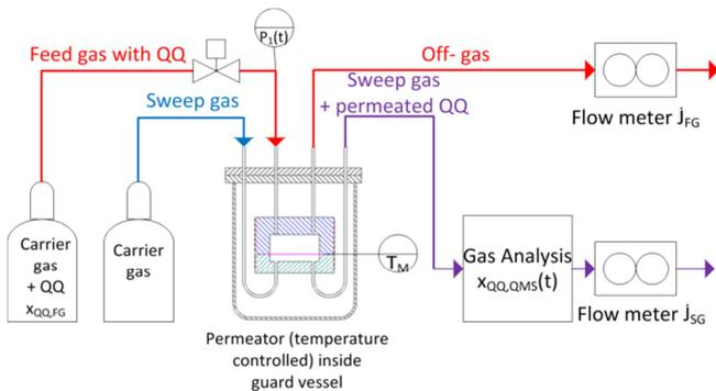
Fig. 1. Functional schematic of the Q-PETE experimental setup
