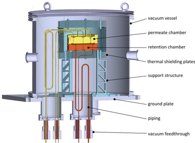
Fig. 3. Guard vessel with permeator inside.
