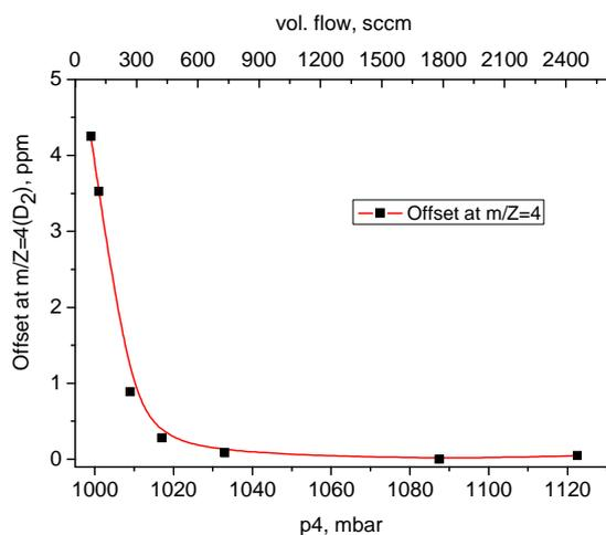
Fig. 7. Signal background at  $m/Z=4$  as a function of pure argon 6.0 volumetric flow (top axis) and inlet pressure  $p_4$  (bottom axis) in preparative experiments.
