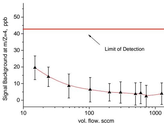
Fig. 9. Signal Background (with average absolute standard deviation for each measuring point) at  $m/Z=4$  vs. volume flow for  $p_4=1.4$  bar (SEM 1400 V).
