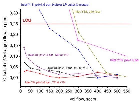
Fig. 8. Signal background at  $m/Z=4$  vs. volume flow for different configurations of the gas inlet of the mass spectrometer (SEM 1200V).
