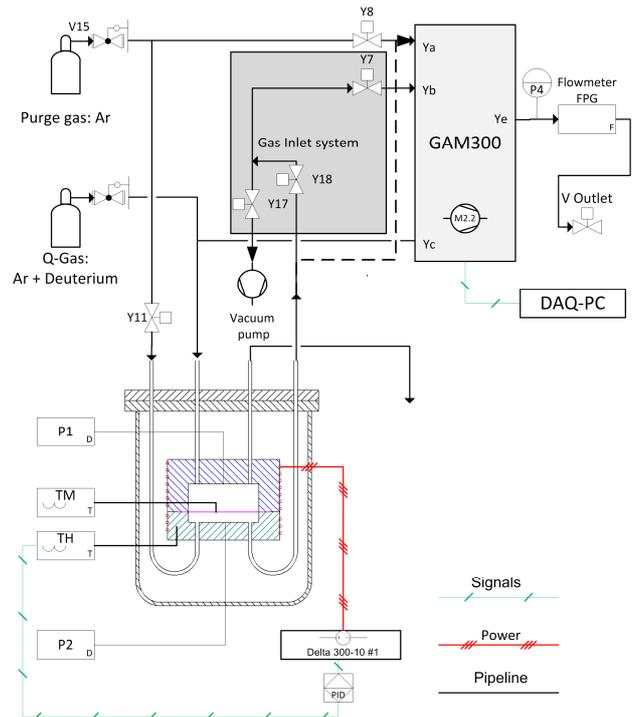
Fig. 5. Process diagram of the PETE-Q setup including the GAM 300 mass spectrometer.
