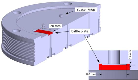
Fig. 4. Cut view of the permeator flange (retentate side).
