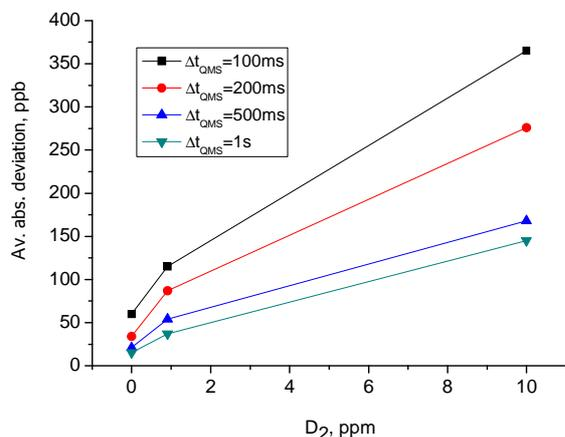
Fig. 6. Average absolute standard deviation at  $m/Z=4$  vs.  $D_2$  concentration. Volume flow: 330-340 sccm. Dwell time:  $\Delta t_{QMS}=1s, 500ms, 200ms, 100ms$ .
