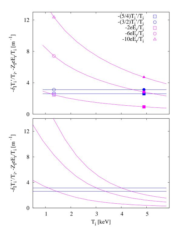
FIG. 5: Convective terms in the impurity flux as a function of the ion temperature. Open and closed signs correspond to the ion root and impurity hole plasma respectively. Scan with  $T_i > T_e$  (top) and  $T_i = T_e$  (bottom).
