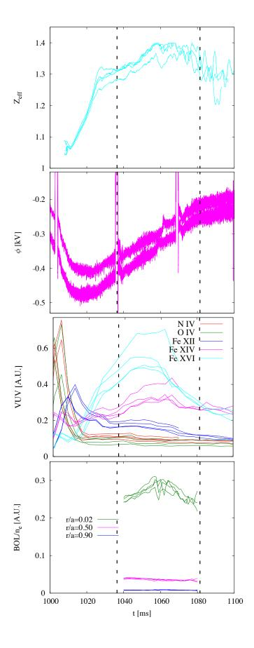
FIG. 9: Time traces for TJ-II discharges #41706, #41709-41711, from top to bottom: effective charge, core plasma potential, total emission from several impurity ions, and central and edge radiation (from tomographic reconstruction of bolometry signal) normalized by the average density. Vertical lines indicate the TS time.
