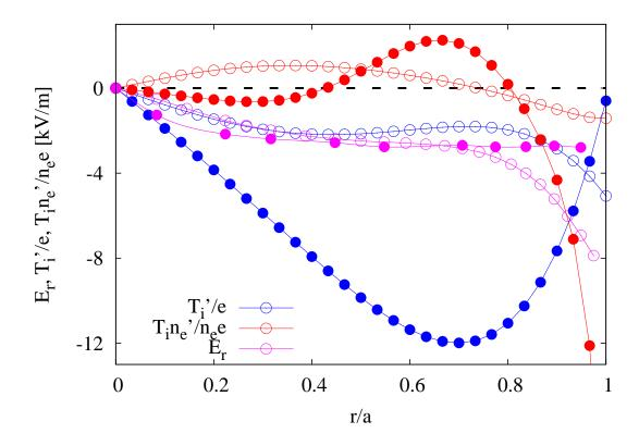
FIG. 4: Ion temperature gradient and calculated radial electric field of LHD discharges #109696, at t=4.440 s (open circles) and #113208 at t=4.640 s (closed circles).
