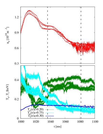
FIG. 6: Time traces for TJ-II discharges #41706, #41709-41711: (top) line-averaged density, (bottom) central and edge electron temperature and central ion temperature.
