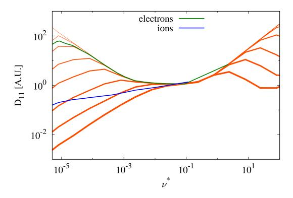
FIG. 3: Monoenergetic transport coefficient  $D_{11}$  (see [11]) at r/a = 0.3. Different orange lines correspond to different values of  $|E_r|/v$ , v being the particle velocity, and thicker lines indicating larger  $|E_r|/v$ .
