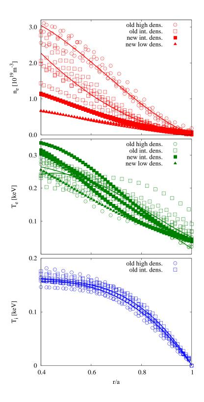
FIG. 7: Density and temperature profiles of TJ-II discharges for high density (open circles), intermediate density (open squares), new discharges with intermediate density (closed squares) and low density (closed triangles).
