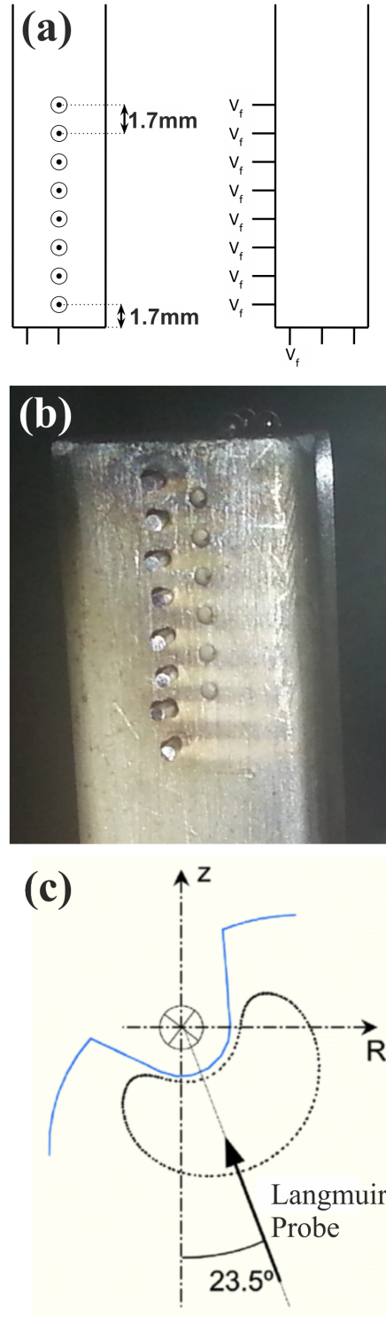
FIG. 3. Langmuir probe: (a) Schematics of the probe system. (b) Recent photograph of the rake of pins. (c) Plasma access region.
