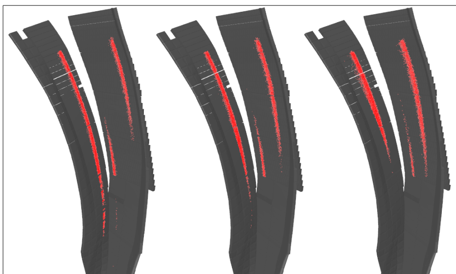
Fig. 5: Effect of different net-currents on magnetic configuration visible by footprints of field lines on vertical and horizontal targets. As previously from left to right: I_{pl} = -3.43kA, 3.43kA, 10.29kA .
