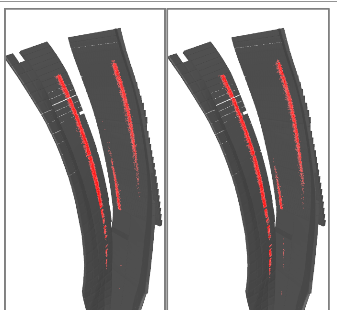
Fig. 9: Comparison of footprints of field on divertor resulting from VMEC/EXTENDER-calculation (left) and from HINT2 (right).
