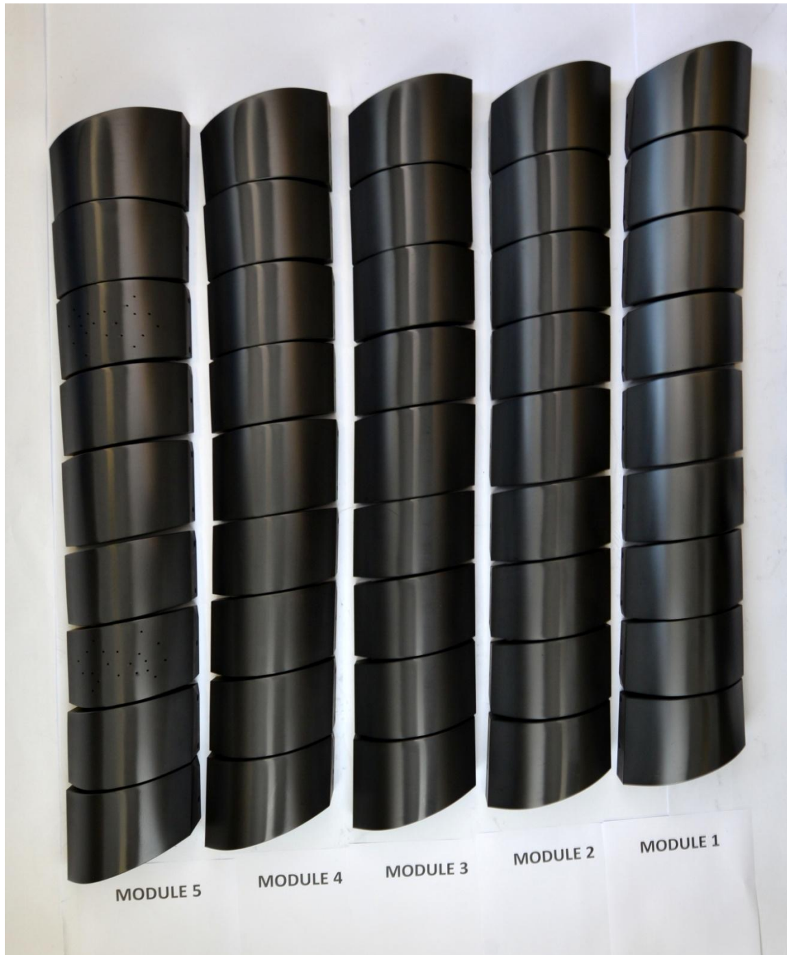
Figure 6. Poloidal (top-bottom) asymmetry on all five limiters. Erosion/deposition patterns stop before the top tile, (with a small curvature to the right), but extend straight off the bottom tile, (with a small curvature to the left).
