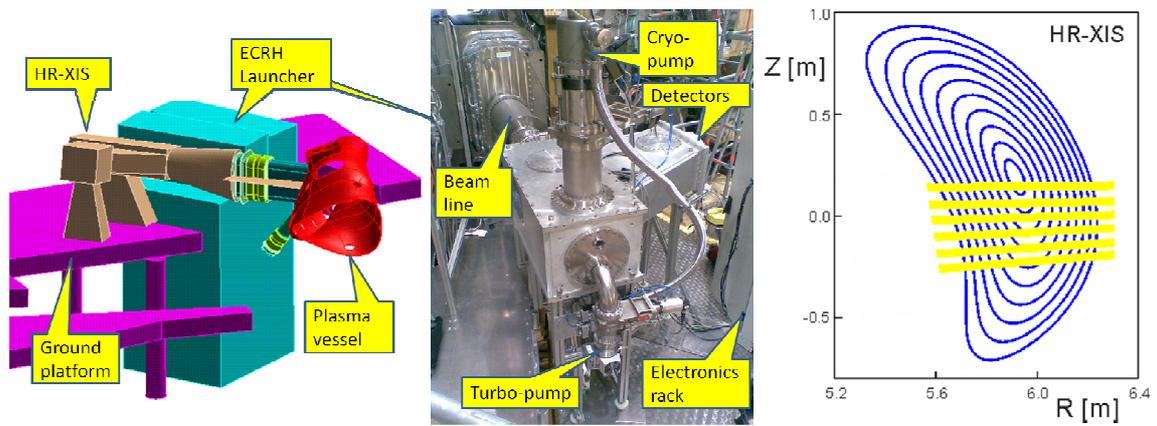
Fig. 2: The installation location in an overview CAD model (left), photo after installation in March 2015 (middle) and the sight lines in the plasma cross-section (right).
