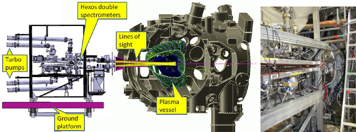
*Fig. 4: Sketch of the central lines of sight of the HEXOS double spectrometers. The plasma contour is shown in blue color.*
