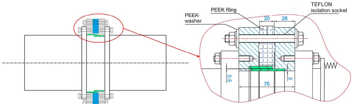
*Fig. 1: Electrical isolation break inside the beam line between two CF flanges. The compatibility with the microwave stray radiation requirements are met by the steel labyrinth housing (green colored), which shields the radiation from the PEEK sealing.*
