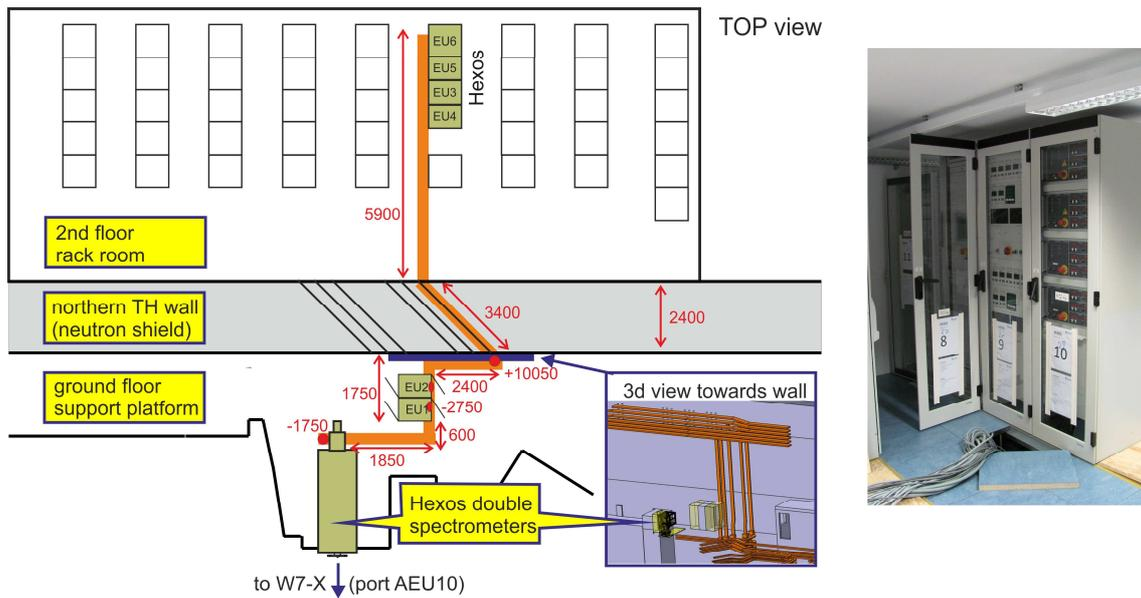
Fig. 5: Sketch (top view) of the torus hall and neighboring rack room behind the torus hall wall. The HEXOS double spectrometers and rack locations are colored in blue. The cable routing paths are shown in orange, changes in height are marked by red circles (red numbers indicate distances in mm). The small inset shows the 3d situation in the torus hall (CAD) with cable trays (orange).
