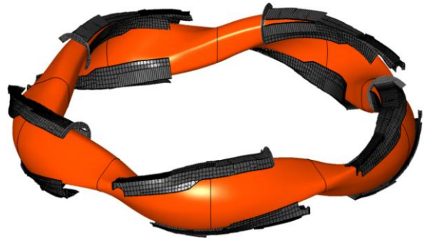
Fig. 2: Plasma contour (orange) with (a) 5 inboard limiters made of graphite (black stripes) defining the last closed flux surface. Fig. 2(b) shows the ten divertor units with the target plates following the topology of the resonant magnetic island divertor.
