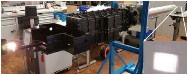
Fig. 8. First optical test with light source (left) produced a focussed image on a screen (right).
