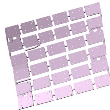
Fig. 1: CAD model of the cooling structure module of a heat shield. The size is approx. 650 x 600 mm 2 . On each of the single heat sinks (approx 100 x 100 mm 2 ) graphite tiles had to be installed
