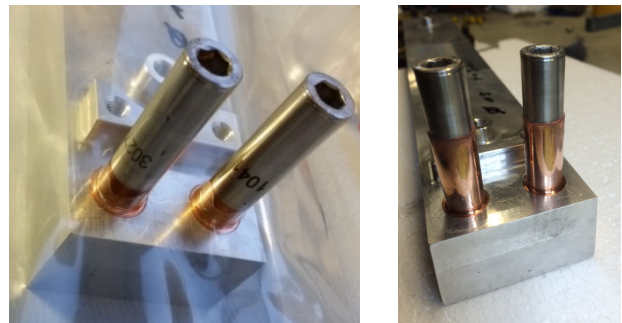
Fig 3: test connectors mounted on dummy Al target element before (left) and after coating (right)
