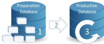
Fig. 2. Manage configuration enhancements at W7-X: 1 – Prepare and test configuration changes, 2 – Release configuration to productive environment, 3 – Adapt existing segments and experiment programs to new configuration
