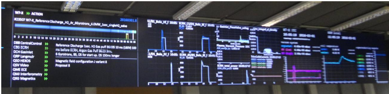
Fig. 4. Xcontrol monitor (left) and DataMonitor on the W7-X control room's video wall
