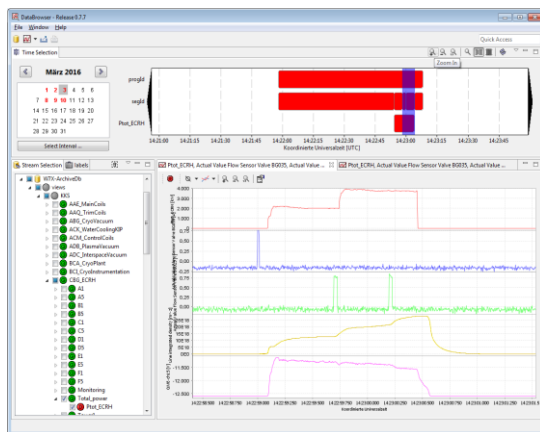
Fig. 5. DataBrowser: Browse data by experiment program time intervals and signal address paths
