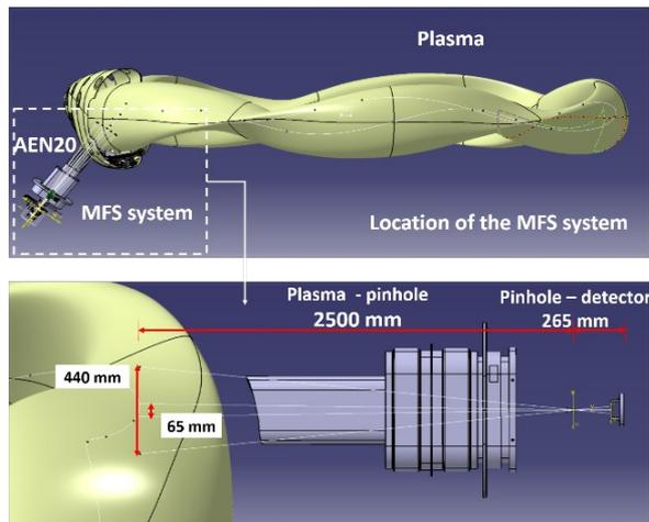
Fig. 2. Localisation (upper figure) and geometry (lower figure) of the MFS system design for W7-X.
