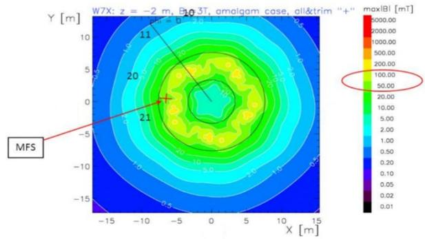
Fig. 5. Position of the MFS system at the magnetic field distribution around the W7-X.
