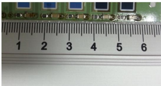
Fig. 1. A single detector array as proposed for the MFS system for W7-X.
