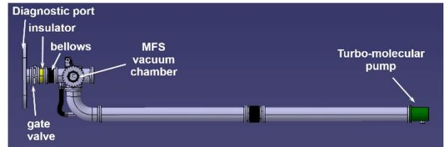
Fig.6. A CAD model of the vacuum pump located at the long distance from the plasma.
