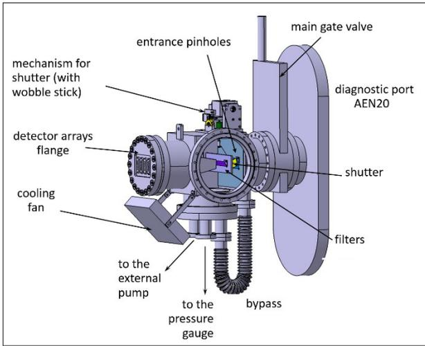
Fig.3. CAD model of the main MFS vacuum chamber.
