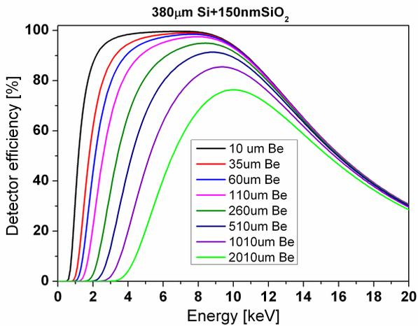
Fig.4. Detector efficiency for 8 MFS detector arrays proposed for MFS dedicated to W7-X.
