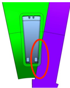
Fig. 12 Interference with the vertical lower port and the poloidal field coil
