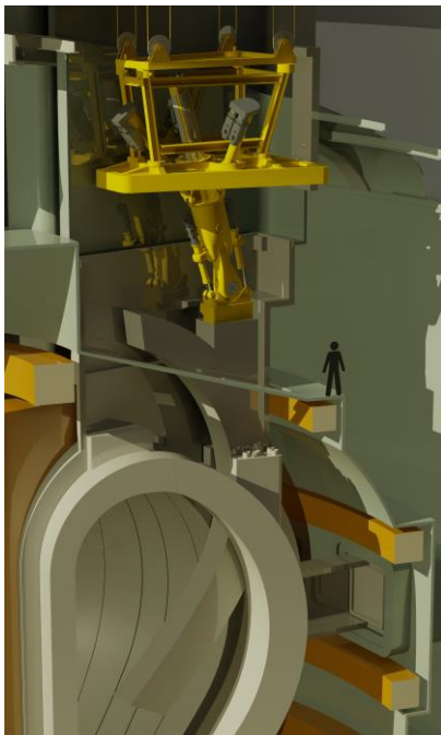
Fig. 1. Section through the 2017 EU DEMO configuration showing the Blanket Transporter removing a blanket.
