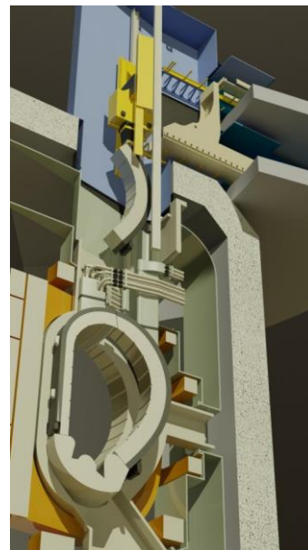
Fig. 1: Vertical port blanket extraction handling scheme
