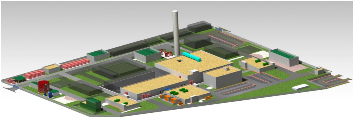
Figure 20. Preliminary layout of DONES in the Granada site (grey buildings are the ones required for a possible future upgrade to IFMIF performance)
