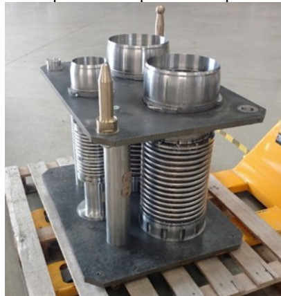
Figure 12. Pipe alignment proof-of-principle pipe module side test assembly
