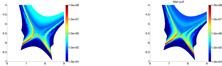
Figure 5: Radiation maps ( MW/m^3 ) in the X-point region. Left: pellet-like injection. Right: neutral puff
