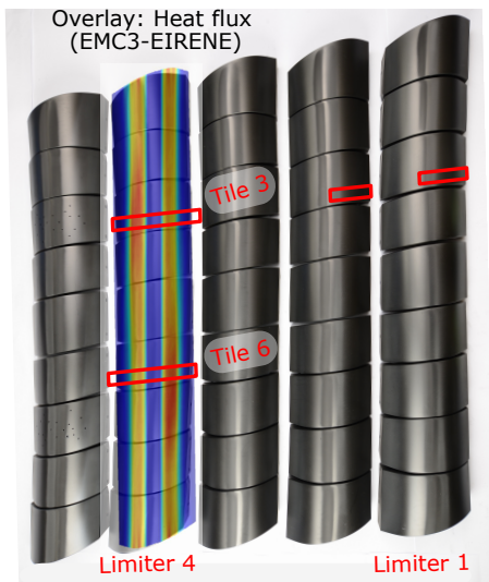
Figure 1: Photo of limiter modules 5 to 1 (left to right), each containing nine tiles. Analyzed tiles are marked in red. On limiter 4 a simulation of the heat flux (EMC3-EIRENE code) owing to electron and ion impact is overlaid.
