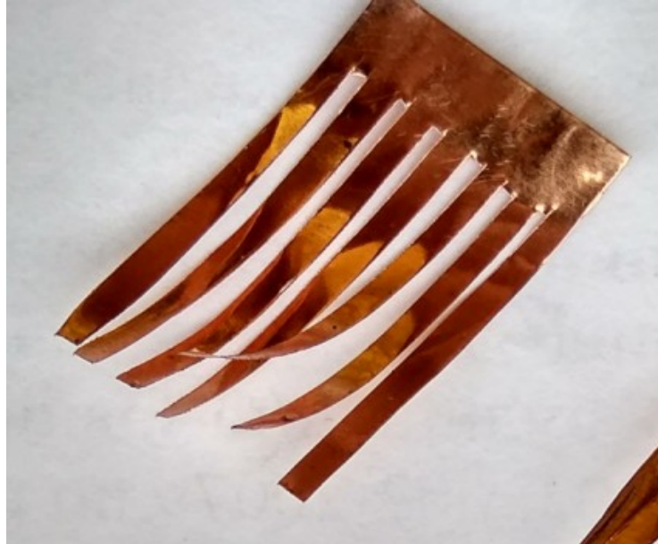
Figure 5. View of electrical shield
