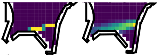
FIG. 7. Example case where the single-ray path terminates too early on a tile surface. When the volume ray-tracing technique is used a large fraction of the collection volume extends into the inner divertor resulting in a significant error in the collected power calculation.
