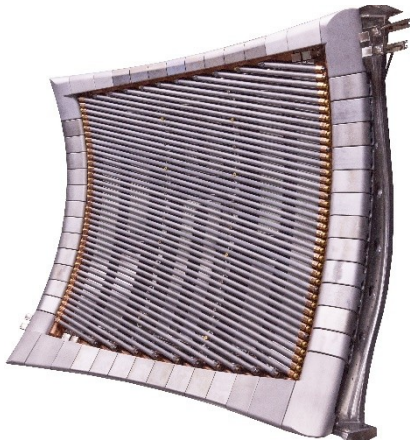
Fig. 3. Real antenna model installed on AUG
