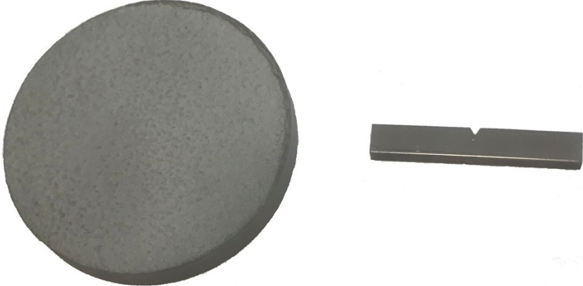
Figure 2 Left: typical sample after sintering; right: the mechanical testing sample
