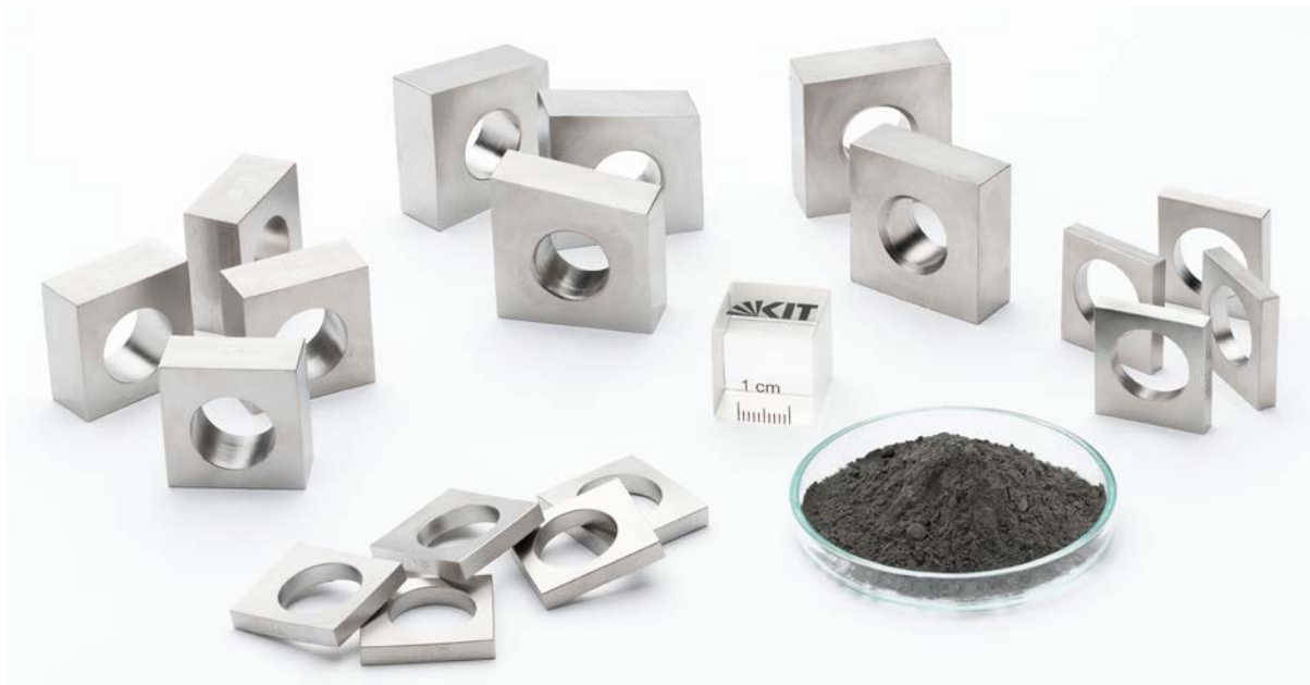
Figure 1. Monoblocks in manifold designs produced via W-PIM. Chamfer (with or without), position and size of bore (center or outboard), thickness (thick or thin) - all these parameters may be varied within certain limits by the use of an adaptable PIM tool.
