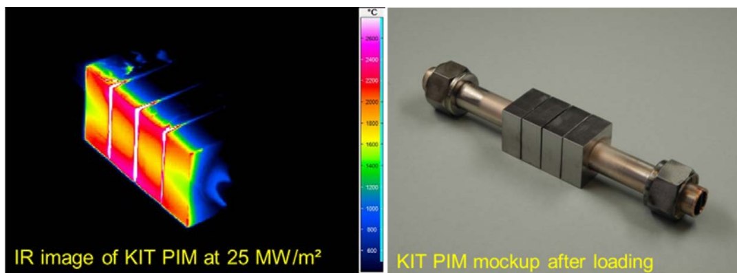
Figure 5. Infrared (IR) image of the mock-up during the screening.
