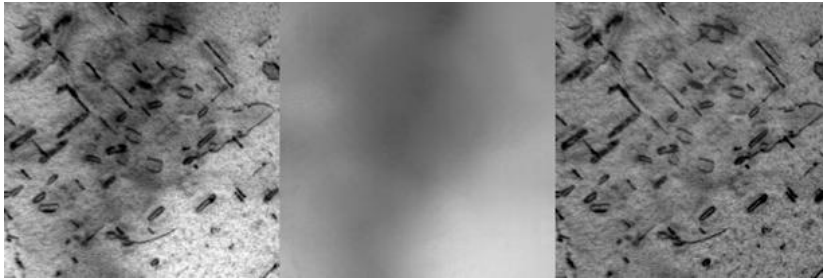
Figure A.5: TEM image background removal. Bright-field image of Fe-9Cr irradiated to 1.8dpa at 350C. Left: original image with varying background. Centre: computed background signal. Right: image with background subtracted. Image courtesy Jack Haley, Oxford University.
