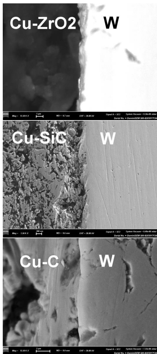
Fig. 7. Microstructure investigation of W-thermal barrier joints produced by FAST: top Cu-ZrO 2 (55% vol.); middle Cu-SiC (50% vol.); bottom Cu-C (65% vol.).
