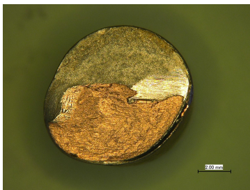
Fig. 11: View on crack position after shear testing
