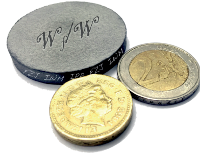
Figure 3: W_f/W produced by FAST with random distributed fibre and 2.5 \mu\text{m} and yttria interface between fibres and matrix
