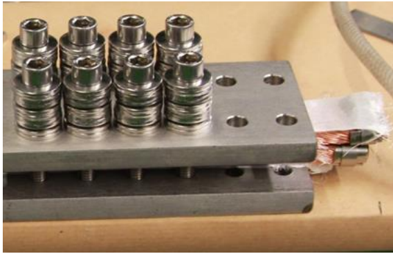
Fig. 7. Clamping fixture made of stainless steel plates, bolts and disc springs
