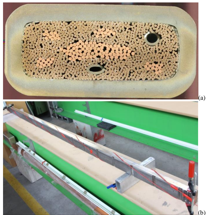
Fig. 1. Pictures of the CICC sample tested in SULTAN in 2016: (a) cross section and (b) whole sample length. In (b) the red markers following the two holes twisted path are also visible (see the text).
