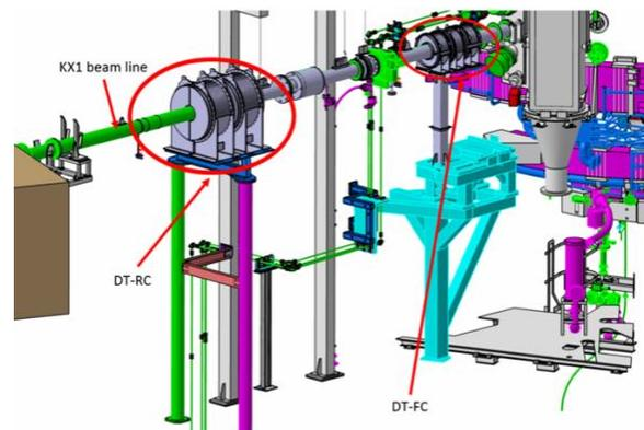
Fig. 1. Upgraded KM6T tandem collimators
