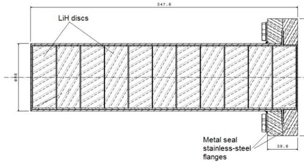
Fig. 8 Cross-section showing the structure of a neutron attenuator
