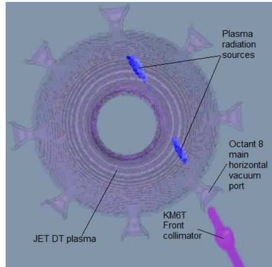
Fig. 9 JET plasma radiation sources for the KM6T tangential gamma-ray spectrometer
