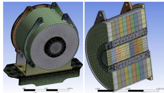
Fig. 4 Complete assembly (for installation); Section of operating assembly (MGRS, sleeve and NA)
