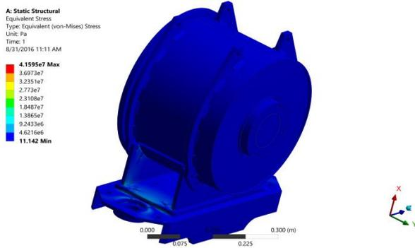
Fig. 5 Stress levels for 42 MPa operation
