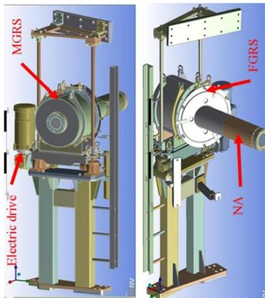
Fig. 2 RFCA components inside the KX1 bunker
