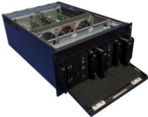
Fig. 1. 5U rack unit containing four acquisition systems.
