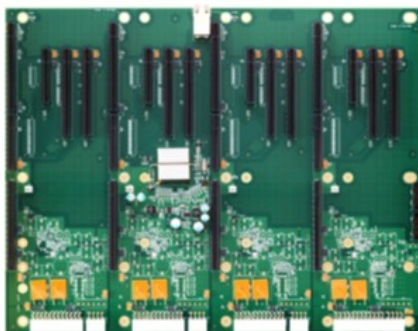
Fig. 2. 4 slot backplane, hosting the acquisition and processing units.
