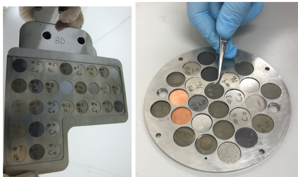
Figure 1: (LHS image) LTIS assembly using on 2015-16 campaign prior to installation and irradiation; (RHS image) New LTIS assembly sample holder containing ITER materials and dosimetry foils prior to installation into JET in 2018.
