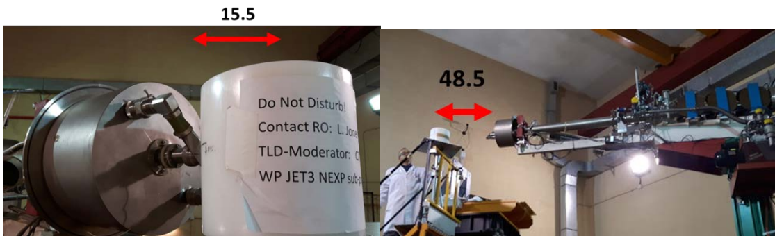
Figure 5. Pictures of the experimental assembly during irradiation in polyethylene moderator at FNG (two positions are shown).
