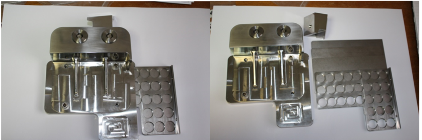
Fig.12 One of the 2 sample holders of the Long Term Irradiation Station (LTIS) to be installed in JET Oct.4 & 8
