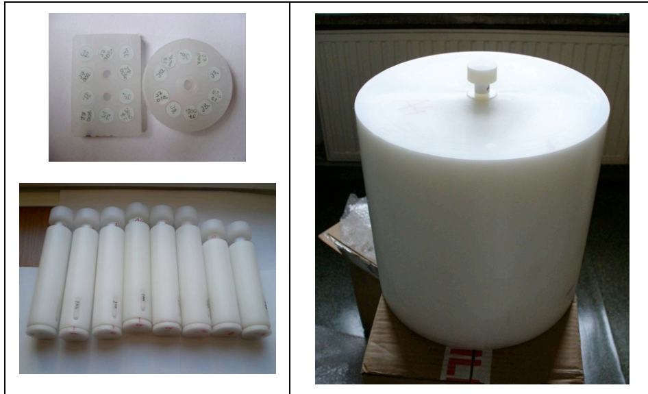
Fig. 6. Left top: The PE-HD boxes with TLDs in place. Left bottom: Some of the plugs with detectors' boxes mounted. Right: The Cylindrical Polyethylene moderator.
