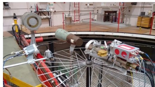
Fig. 2 NPL lower scatter cell with NG, DePangher long counter and shadow cone.
