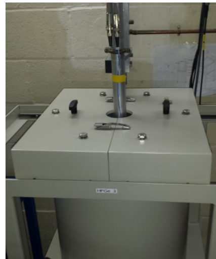
Fig. 3. KN2 transfer system at the counting station . Capsule inside the tube entering the lid of the low background lead shield to the detector within.
