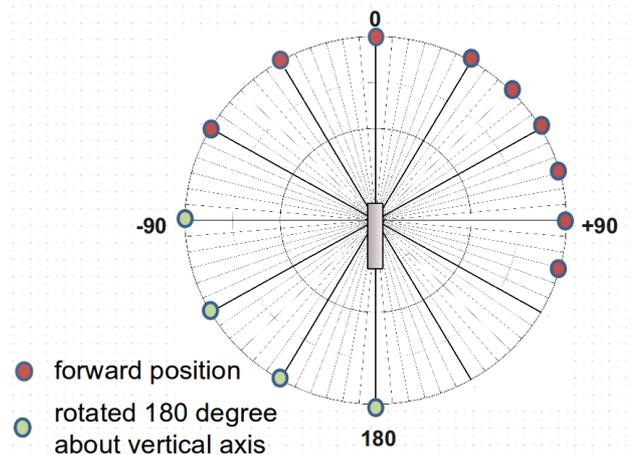
Fig. 3: Measurement positions of the NE-213 detector.
