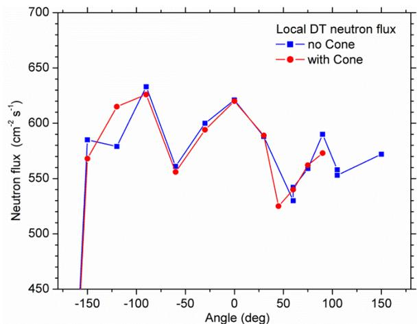
Fig. 8: Neutron flux densities at 14 MeV (DT) at different angles with respect to the CNG axis.
