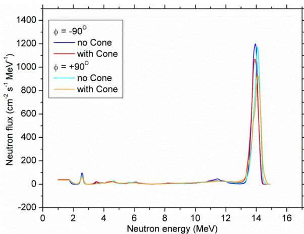
Fig. 6: Neutron spectrum at the 90 degree positions. Note that the DT neutron peak position is shifted towards lower energies as compared to the 0 degree position in Fig. 4.
