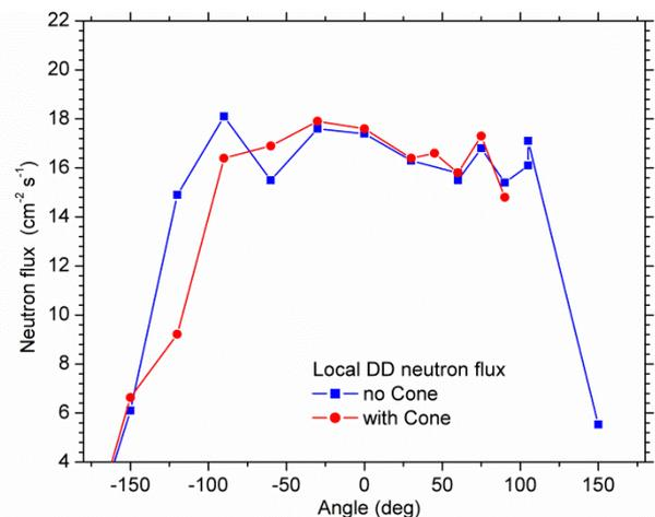
Fig. 7: Neutron flux densities at 2.5 MeV (DD) at different angles with respect to the CNG axis.
