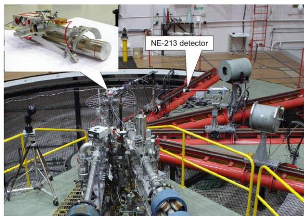
Fig. 1: The compact neutron generator and the set of neutron detectors setting at NPL.
