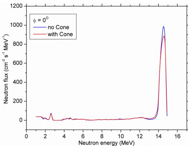
Fig. 5: Neutron spectrum at the 0 degree positions.
