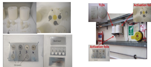
Fig. 3 Activation foils in polyethylene moderator (top-left) and aluminum holder (bottom-left) and assembly of TLDs and Activation foils in position A2 (right) [11].
