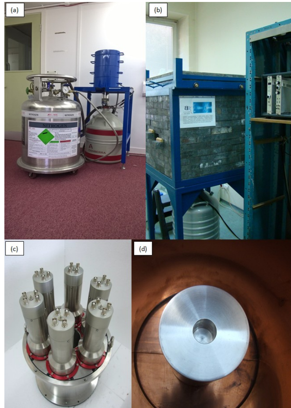
Figure 6: (a) IFPiLM HPGe detector and lead shielding; (b) IFJ PAN HPGe detector and lead shielding; (c) CCFE BEGe detector with NaI Compton suppression ring; (d) CCFE SAGE well detector.
