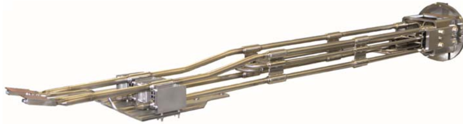
Fig. 7, A two-arm prototype pneumatic shutter for the core CXRS diagnostic
