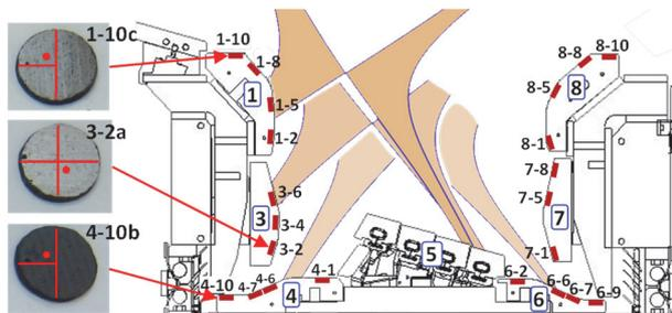
Fig. 1 Poloidal cross-section of the JET ILW divertor with three representative plasma geometries [12], and positions of all samples. Photographs of three analyzed sample are shown in a left side row. Lines and symbols in photographs are the cutting tracks and the analyzed positions, respectively.
