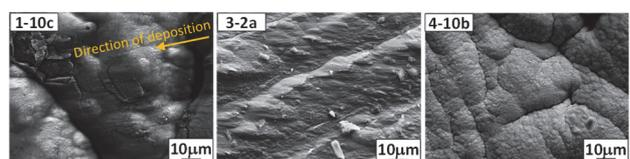
Fig. 2 SEM images of 1-10c, 3-2a, and 4-10b samples. Incident direction of the deposited elements in 1-10c shown by an arrow in the image.
