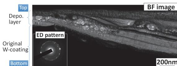
Fig. 4 Cross-sectional BF-TEM image of 1-10c sample and corresponding ED pattern from the deposition layer.
