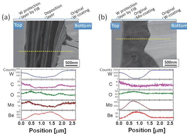
Fig. 3 Cross-sectional SEM images of (a) 1-10c and (b) 3-2a sample fabricated by FIB, and corresponding element profile of W, C, O, Mo and Be along with a dashed line in each SEM image. W protection layers were artificially created on the top surface of the each sample by FIB.
