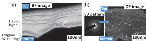
Fig. 6 (a) Cross-sectional BF-TEM image of 4-10b sample. (b) ED pattern of the mixed-material deposition layer and DF-TEM image obtained from a part of the Debye ring as drawn in the white circle region in the ED pattern.
