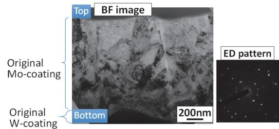
Fig. 5 Cross-sectional BF-TEM image of 3-2a sample and corresponding ED pattern from the original Mo-coating.
