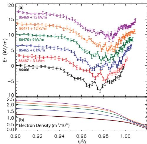
FIG. 3. (Color online) (a) Ohmic  $E_r$  profiles for six shots at different densities,  $t=12.4-12.6$  s. For clarity, for each density increment the  $E_r$  profile is offset by an additional 3 kV/m (annotated). (b) Averaged  $n_e$  profile 12.4-12.6 s, from a profile reflectometer.
