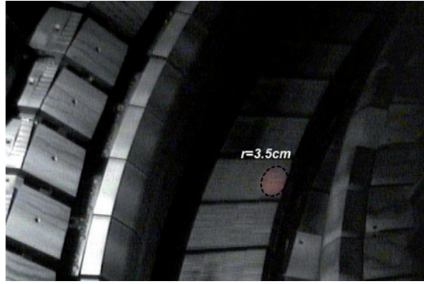
Figure 6: Backlit observation volume for the local W spectroscopy.
