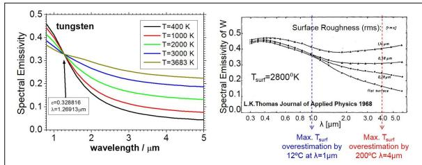
Fig. 3. (left) W spectral emissivity according to [12] and (right) the normal spectral emissivity of W with different surface roughness in dependence of wavelength [14].
