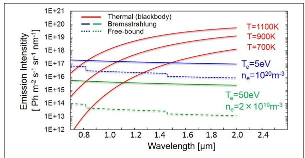
Fig.1 Calculated continuum emission spectrum contributions from Bremsstrahlung, radiative recombination and thermal emission for a 2 m thick isotropic deuterium plasma
