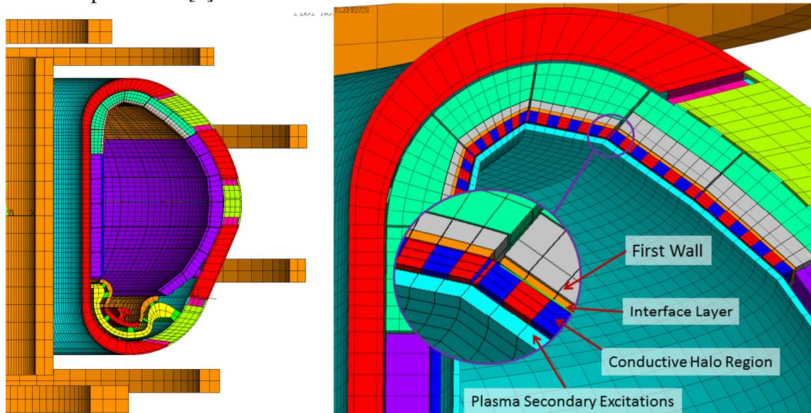
Figure 2 – Left: section of the conductive components included in the ITER tokamak 360 degrees Ansys FE model; right: details of the machine top
