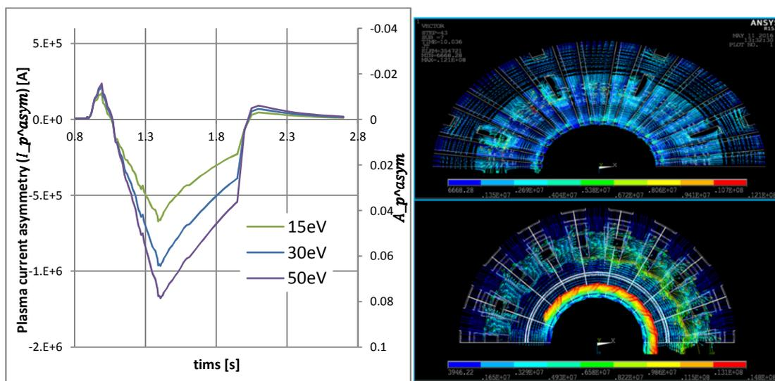
Figure 4 – Left:  $\Delta I_p$  and normalised plasma current asymmetry ( $A_p^{asym}$ ) during locked upward slow AVDEs with a plasma temperature across the gaps of 15, 30 and 50 eV. For all simulations the thermal quench is at 885 ms. The asymmetry is triggered at 900 ms and lasts until 2000 ms when the plasma has lost about 90% of its original current. Right: The induced current distribution in JET (top) and ITER VV (bottom) during the current quench phase of an upward AVDE.
