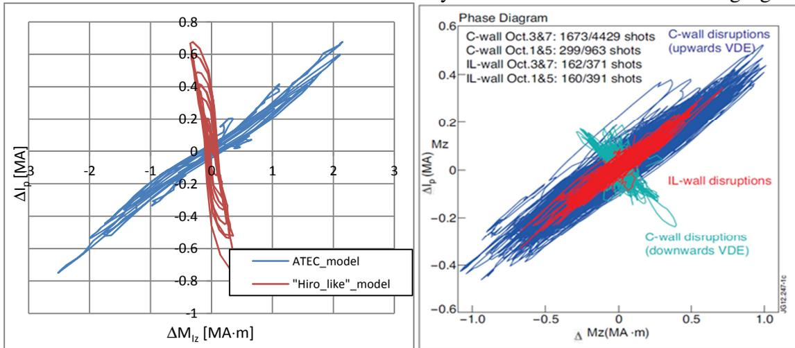
Figure 7 – Measured at JET (right) and calculated applying ATEC model to ITER (left) phase relationship between plasma current ( $\Delta I_p$ ) and first plasma current vertical moment ( $\Delta M_{IZ}$ ) asymmetries. “Hiro\_like” shows how the plot would look in the case of a positive surface current mirrored with respect to the plasma centroid.
