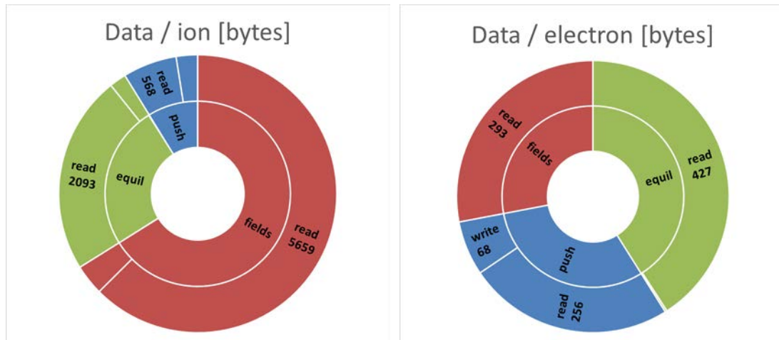
Fig. 34 The amount of bytes read from main memory for different subparts of the particle loop, for the ions on the left and the electrons on the right. The values are per particle. Additionally, each subpart is split into a “read” and “write” value.
